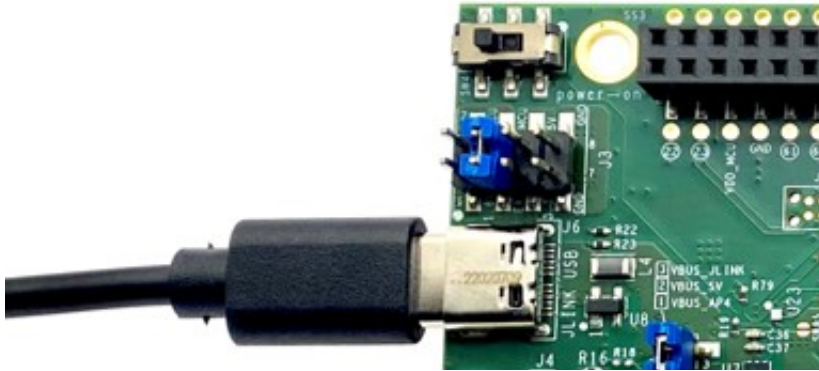
Figure 6. Apollo4 Lite EVB - Using On-board J-Link Debugger
