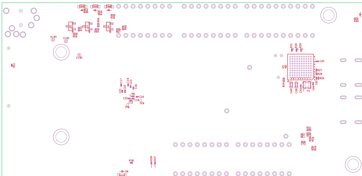
Figure 4. Apollo4 EVB - Bottom-side Parts Location
