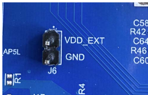
Figure 12. J6 External Supply Header
