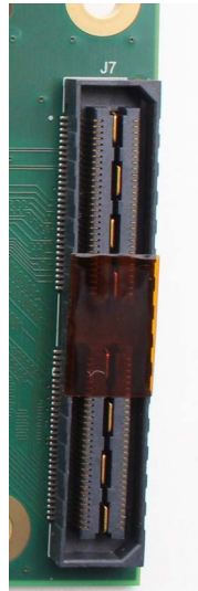
Figure 9. Board View of J7 High-speed Header
