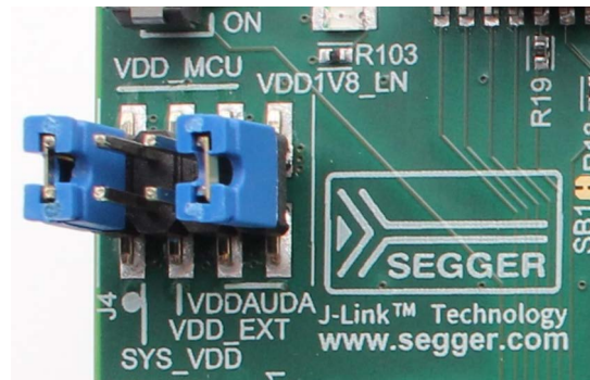
Figure 14. J4 Default Jumper Configuration
