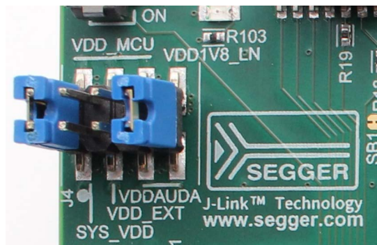
Figure 14. J4 Default Jumper Configuration
