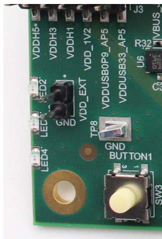
Figure 12. J6 External Supply Header
