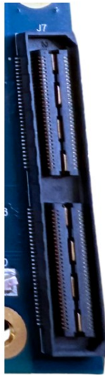
Figure 9. Board View of J7 High-speed Header
