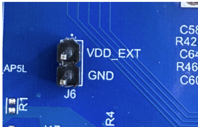
Figure 12. J6 External Supply Header
